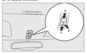
Press the switch  $\blacksquare$ , and the sunroof will close while the switch is pressed.
