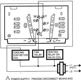
POWER SUPPLY. PROVIDE DISCONNECT MEANS AND OVERLOAD PROTECTION AS REQUIRED. M2412
