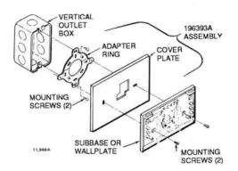
Carefully level the wallplate or subbase and firmly tighten screws.
