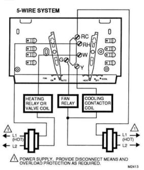
NOTE: If there are four wires, connect wire marked R to terminal RH and add a jumper wire to connect to RC. If RC is left unconnected, the air conditioner will not turn on. The 4-wire drawing on this page shows how to jumper RC to RH. Strip the insulation off the wire where it connects to the terminals. Firmly tighten screws.
