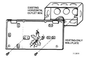
If mounting on outlet box, mount as shown on appropriate figure.
