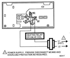
Connect either wire to R terminal and the other wire to W terminal. Firmly tighten screws.
